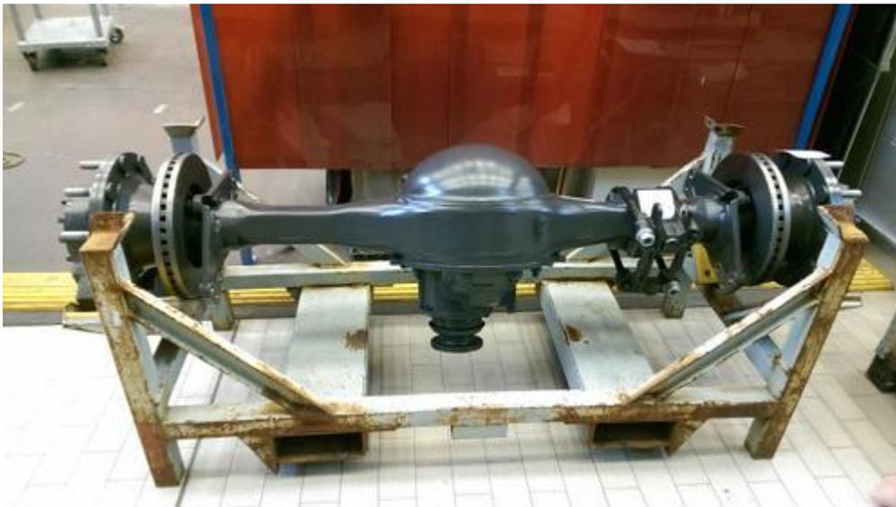
**Figure 3** The drive axle from Meritor to be used together with the electric motor and generator and batteries in the SchmitzCargobull semi-trailer prototype.
